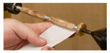
7. Move the tool rest away from blanks and sand the blank through 320 grit then final sand with steel wool.
