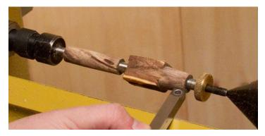
5. Turn the corners off the blank with the Mini Easy Rougher. Start at one end of the blank and work toward the center a cutter-width at a time. Turn both blanks down to a cylinder about 1/8" larger in diameter than the pen bushings.
