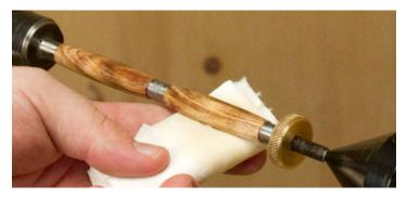
8. With the lathe stopped, apply the first coat of finish. Turn the lathe on and with light pressure buff the blank with the rag. Repeat until desired gloss is achieved. Apply a small amount of wax to a small rag and lightly buff the blanks to a final finish.
