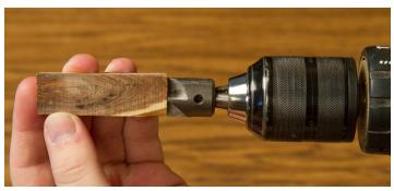
**3.** Trim the ends of the pen blanks using a barrel trimmer. This squares the ends of the blank to the center of the tube assuring a proper fit during assembly.
