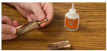
**2.** Glue the brass tubes into the drilled blanks using CA glue or epoxy.
