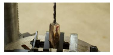
1. Select a pen blank of suitable size, cut in two and drill the required hole through the center of both pieces.
