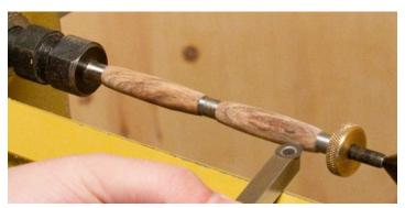
6. Turn the blanks to the finished shape and diameter with a the Mini Easy Finisher. Taper the blank in the direction bushing on each end of each blank, leaving the center slightly thicker.
