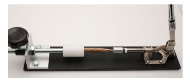
2. Press the writing tip into the end of one barrel.
