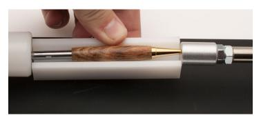
**3.** Start the twist mechanism, brass end first, into the opposite end of the writing tip. Lay the assembly parts into the vee groove of the Pen Press Block and press the parts together until the block stops the parts from pressing together any further.
